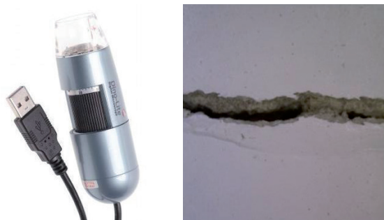
Figure 16. Digital microscopy lens – typical crack image 60 x.
